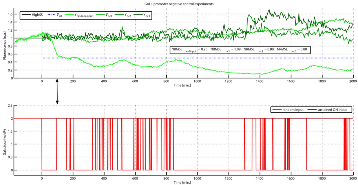
Figure 6. In-vivo negative control experiments on the GAL1 promoter. (Top panel) the three green signals ( y_{nc1} , y_{nc2} and y_{nc3} ) represent the measured GFP fluorescence in the cell population for a constant concentration of galactose. The desired ( y_{ref} in blue) and experimentally quantified GFP fluorescence ( y_{random\ input} in light green) for the whole duration of the random input negative control experiments are also shown. For this experiment, the control action starts at time t=0 and it is stopped at time t=140 min as soon as the GFP reaches the desired set-point (arrow), from this time instant onwards, the input randomly switched between galactose and glucose, as described in the Supplementary Information. (Bottom panel) the dark red line represents the constant concentration of galactose (2%) provided to cells corresponding to the experiments y_{nc1} , y_{nc2} and y_{nc3} ; the light red series of pulses, corresponding to the experiment y_{random\ input} , represents the closed loop control input calculated by the control algorithm starting from time t=0 min up to time t=140 min, as indicated by arrow; from this time onwards, the input randomly switched between glucose and galactose (Supplementary Information). doi:10.1371/journal.pcbi.1003625.g006
