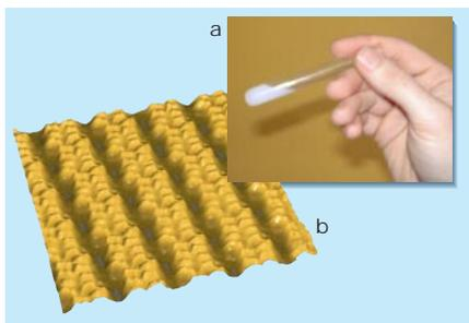
**Figure 2** The dual nature of liquid crystals. **a.** In a bottle the liquid-crystal material looks turbid, owing to the imperfect alignment of the liquid crystal. **b.** Like a solid, liquid crystals can also show surprising amounts of order. Perfect alignment of individual liquid crystal molecules (an alkylated cyanobiphenyl) on a graphite surface, as observed with a scanning tunnelling microscope (J. Gerritsen, Univ. Nijmegen, The Netherlands; see also ref. 8).
