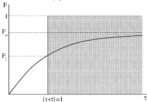
**Fig. 2** Cumulative distribution function of times until the next reaction for case 2 when no time-independent channels are present. If URN  $u_1$  is greater than  $F_1$  (given by (13) with  $\tau = 1 - \{t\}$ ), instead of selecting the next reaction, the cell division at time  $t - \{t\} + 1$  is performed
