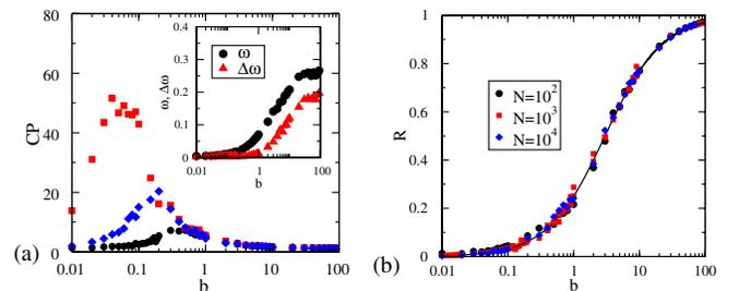
FIG. 2 (color online). Gillespie simulations of coupled stochastic oscillators: coherence parameter  $CP = \Delta\omega/\omega$  (a) and order parameter  $R$  (b) vs.  $b$  for  $N = 10^2, 10^3, 10^4$ . Solid line in (b) is (8). Inset: frequency  $\omega$  and bandwidth  $\Delta\omega$  vs  $b$ .
