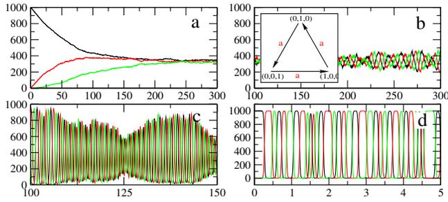
FIG. 1 (color online). Time series of the instantaneous occupation numbers oscillators  $n_1, n_2, n_3$  in states 1, 2, 3, respectively, for  $N = 1000$ , and different values of the coupling parameter: (a)  $b = 0$ , (b)  $b = 0.1$  (Inset: Transition diagram in a single unit); (c)  $b = 1$ , (d)  $b = 10$ .
